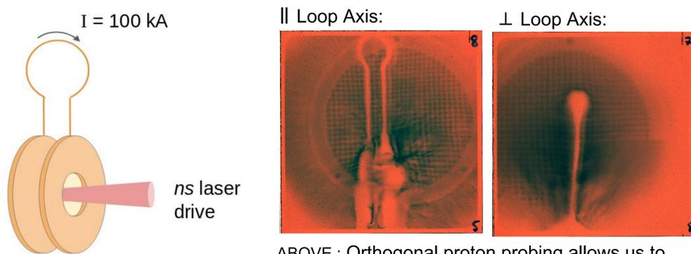
ABOVE : Orthogonal proton probing allows us to differentiate between E and B-fields.
