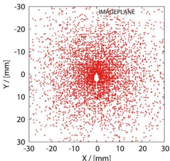
Static field solution for 10 MeV protons passing across a loop with a 10kA current for experimental configuration outlined in [J. Santos, NJoP, 2015].
